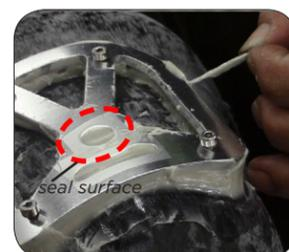
Apply Vaseline to the mating surface of the Side Mount Lamination Dummy.
