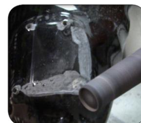
Using a small screwdriver, pry up the corner of the Lamination Dummy. Remove the Lamination Dummy.
