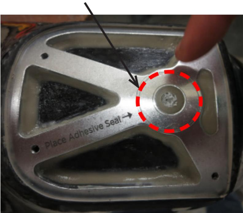
3. Apply the sealing gasket to the LimbLogic Side Mount pump and attach the pump to the socket as described in the *WillowWood One System Socket Fabrication Instructions* booklet.
